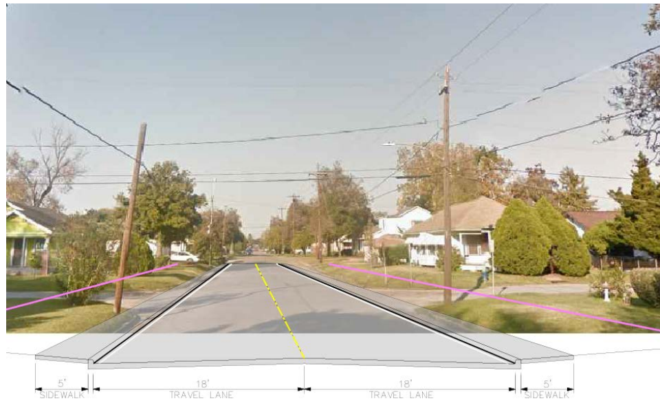
OPTION 2 – 36' WIDTH TYPICAL PROPOSED CROSS-SECTION – STREET VIEW 79TH STREET FROM HUDSON STREET TO HARRISBURG BLVD
