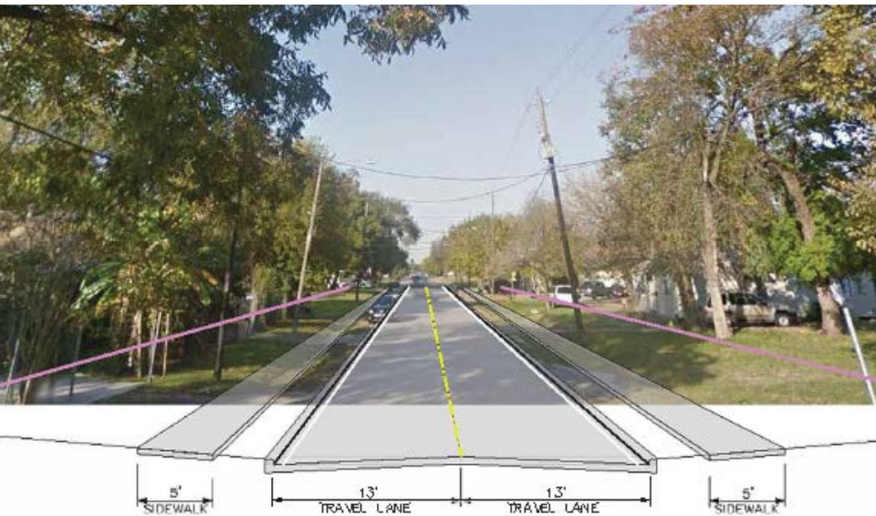
OPTION 1 – 26' STANDARD WIDTH TYPICAL PROPOSED CROSS-SECTION – STREET VIEW 79TH STREET FROM BRAYS STREET TO HARRISBURG BLVD
