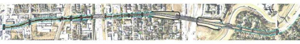
The project will improve approx. 1.5 miles of T.C. Jester Blvd. between Washington Ave. and Timbergrove Ln. improvements include new pavement, improved intersections, new bicycle lanes, and upgraded storm drainage, water & sewer infrastructure.
